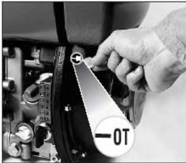
Fig 31 Flywheel cover inspection hole
