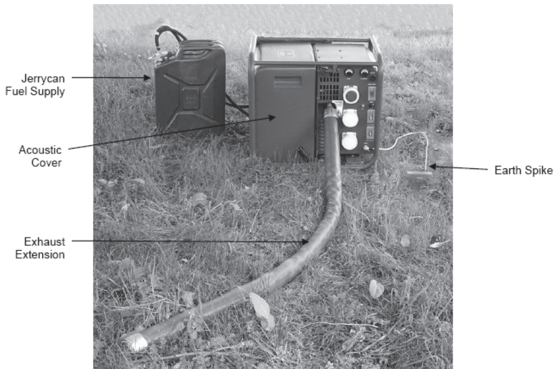
Figure 1 General view of LFG - ready to operate
